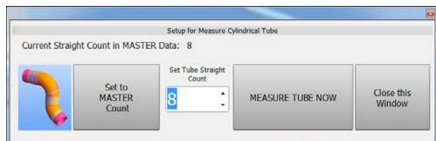
16. Measure the part following the instructions in the guide box like the one shown here. The yellow box tells you the current step.
